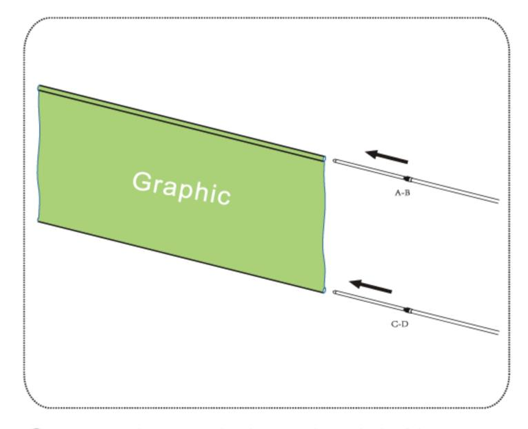
To put pole #A-B and pole #C-D through the fabric 4 To use right number of screw for tightening. banner hem.
