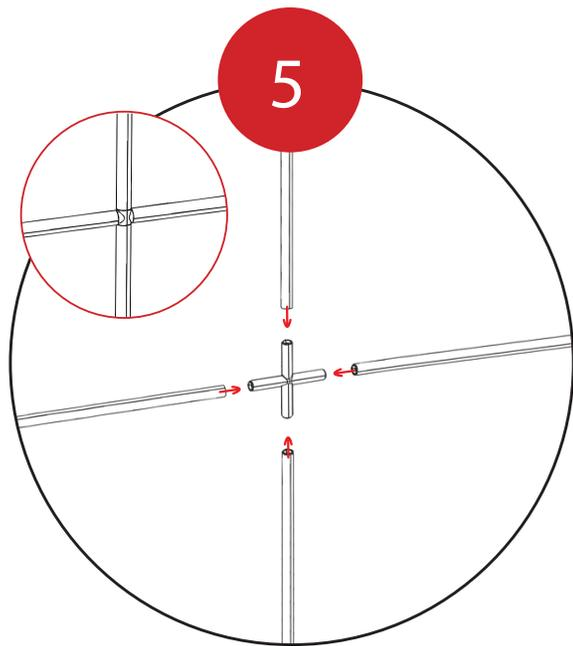
Fit the Channel Bar
