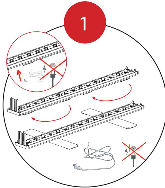
Fit the Bottom Extrusions together.
