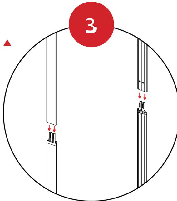
Fit the Top Extrusions together.
