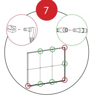
Fit your graphic(s) into the channel on the top and bottom extrusions.
